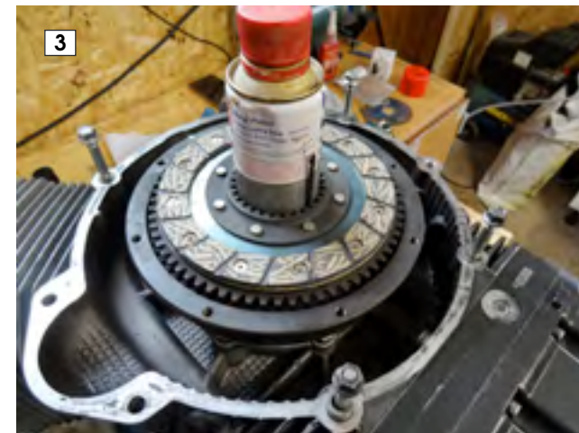
Fitting additional clutch plates
