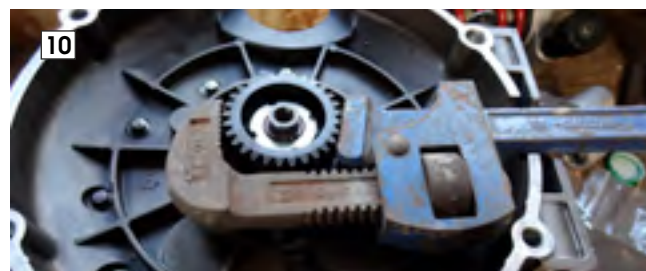
Locking the gearbox spline
