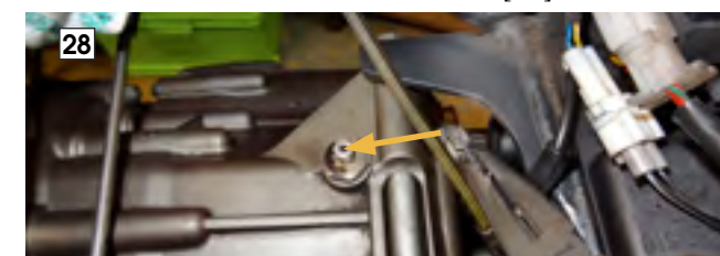
Reconnecting the neutral switch terminal
