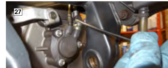
Reconnecting the clutch master cylinder union
