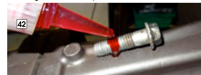
Use Loctite on the drive housing bolts
