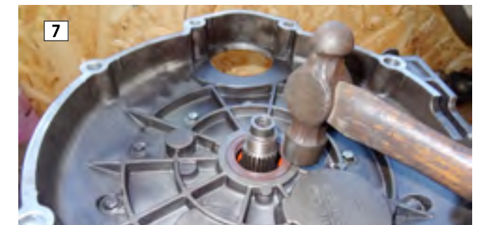
Tapping in the oil seal
