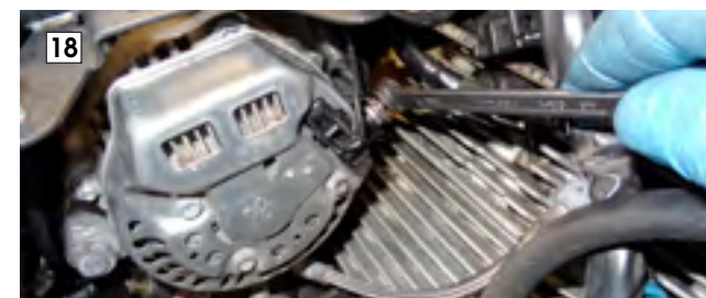
Refit the alternator connections
