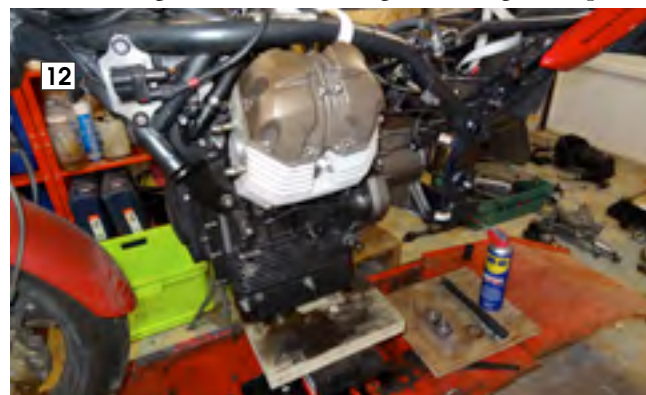
Lifting the engine and gearbox into place
