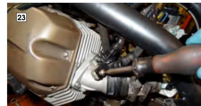
Refitting the injectors
