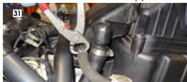
Refitting an oil/air separator pipe
