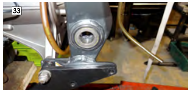
Swinging arm bearings in place
