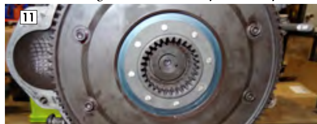
Refit the clutch pushrod centre
