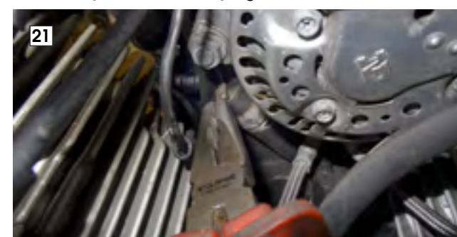
Fitting the oil pressure switch terminal
