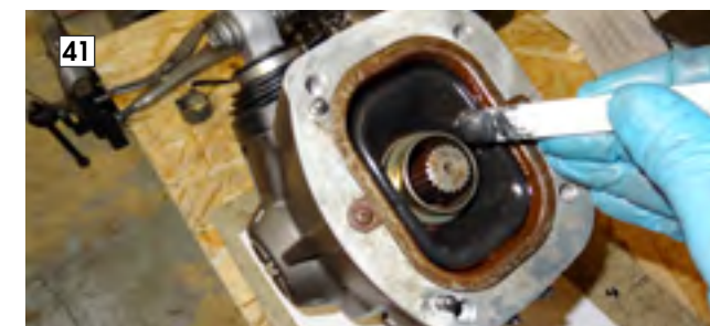
Greasing the final drive spline
