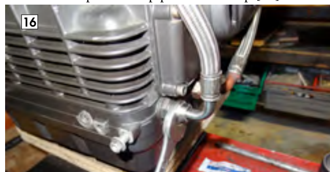
Connecting sump oil pipes
