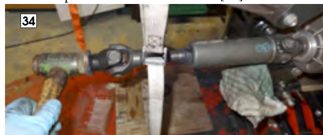
Fitting the driveshaft
