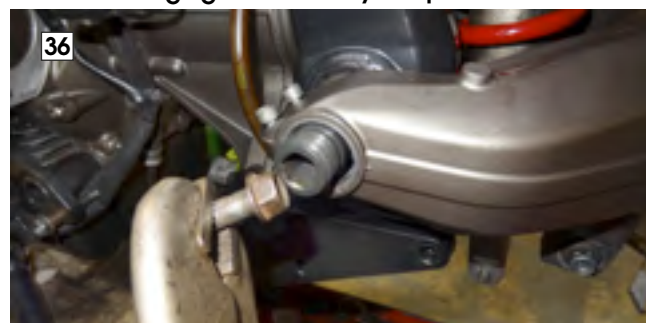
... and tighten the pivot bolt
