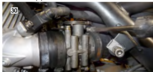
Fitting an inlet rubber
