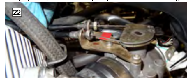
Refitting the throttle cables
