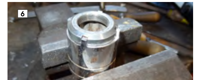
Home-made peg nut socket
