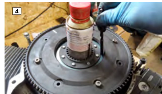
Check with 7mm drill bit while tightening the 25mm bolts
