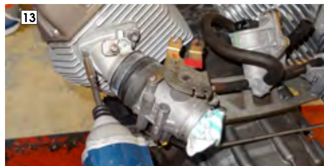
Refitting the injector manifolds
