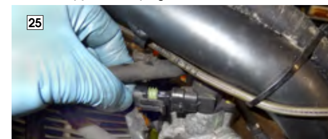
Connecting the TPS plug
